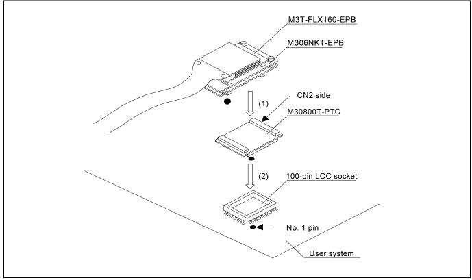
Figure 2.9 Connecting to a 100-pin LCC socket
